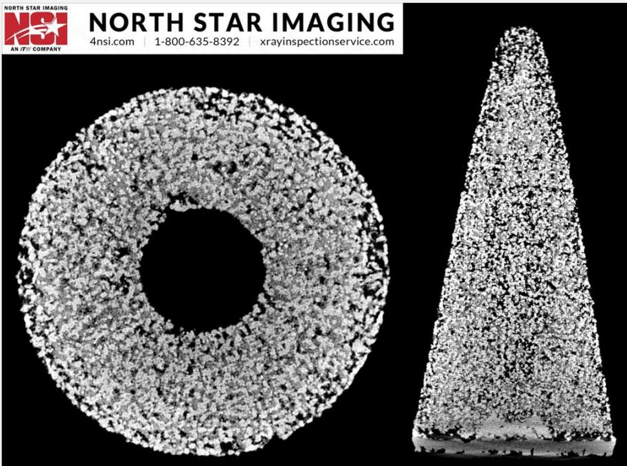
**Figure 3:** X-Ray CT images of the AM porous filter
