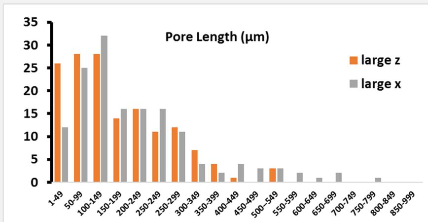
**Figure 4:** Aperture size distribution of SS316L AM porous filter
