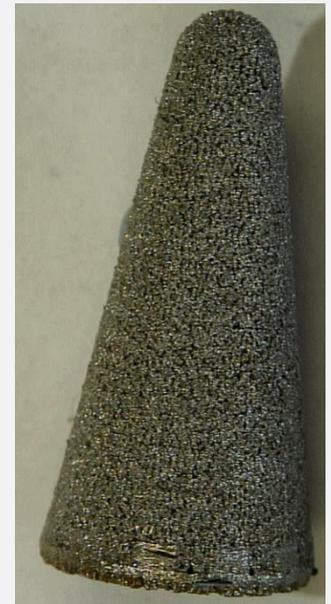
**Figure 1:** SS316L AM porous filter
